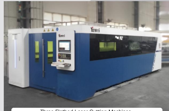
Three Flatbed Laser Cutting Machines (6000W, 4000W, 3000W)
