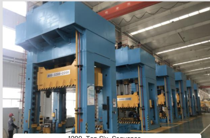
1200-Ton Six-Sequence Stamping Production Line
